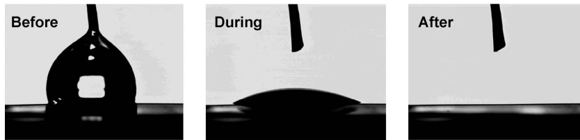
Fig. 8. Photographs of the EC-DMC electrolyte undergoing the electro-wetting transition on the surface of superlyophobic membrane treated with Teflon AF. The duration of the transition is on the order of 1–2 s.
